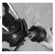
Insert regulator into facepiece adapter by pushing inward.
