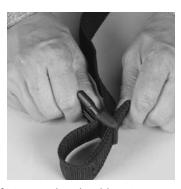
14. Connect the strain relief strap to the shoulder strap snap hook.
