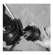
**NOTE:** Regulator can hang on cover rail in a standby mode.
