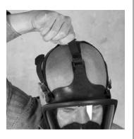
4. Tighten the lower straps first by pulling them straight back, not out. Tighten the facepiece until the mask is snug against the face.
