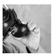
Push the release buttons and pull regulator down and out of facepiece adapter.
